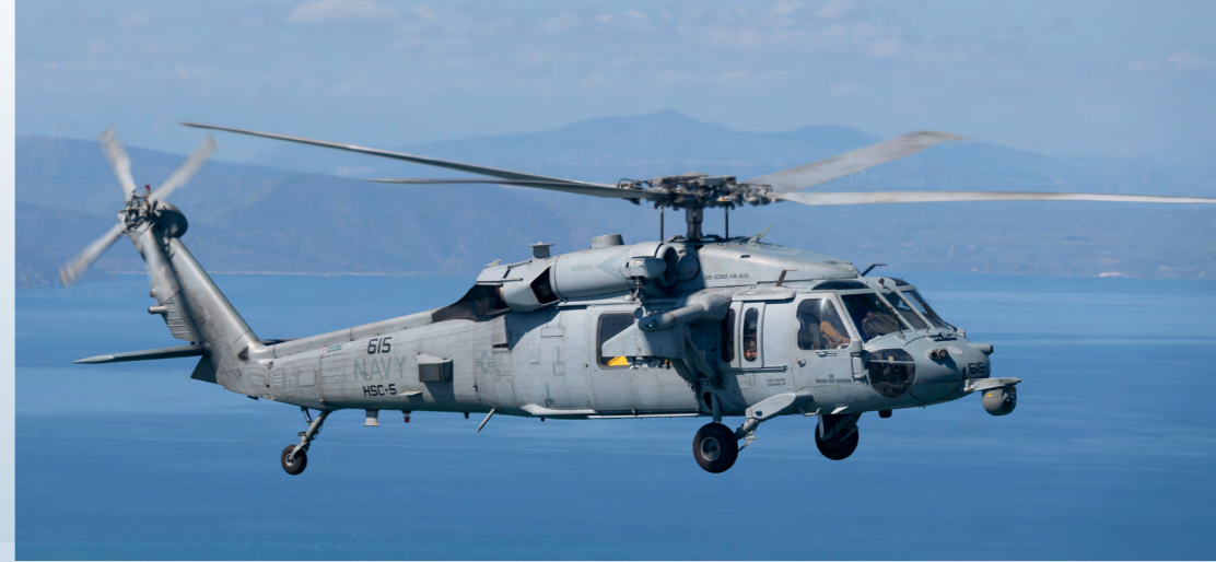
Top Left: The MH-60S Knighthawk fulfills the SAR tasks during operations at sea – it is the first aircraft to take off prior to each mission and the last to return to deck once all aircraft have been recovered
