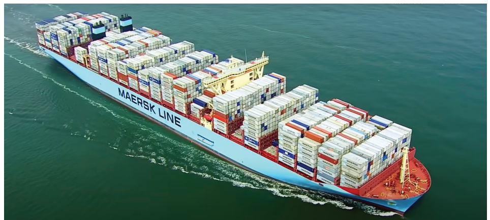
MV Marie Maersk , Triple E-class container ship (1st generation), 196,000 DWT, diesel propulsion, 23 knots max speed, capacity 18,270 TEU, built in 2013, Danish flagged
