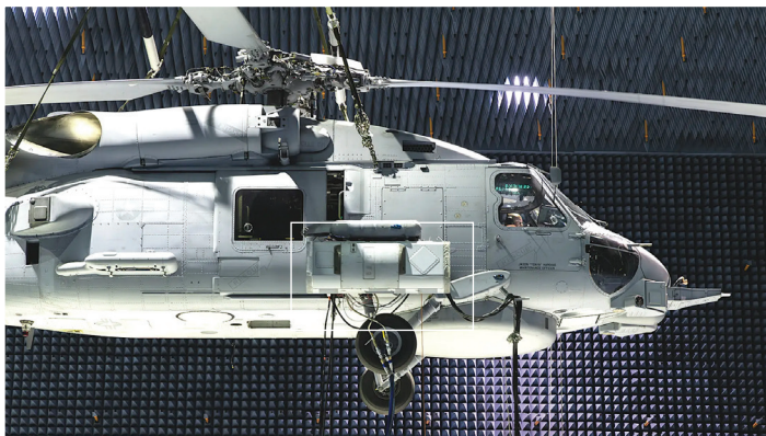
The new pod being tested in an anechoic chamber at Naval Air Station Patuxent River
