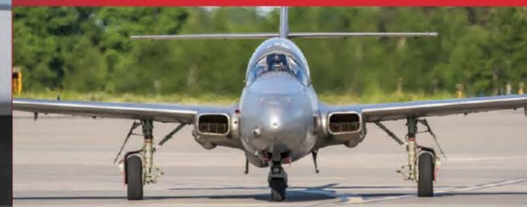
Above: Designed to operate from less than perfect airstrips the TS-11 was equipped with 'mudguards' on the engine intakes Paul Gross
